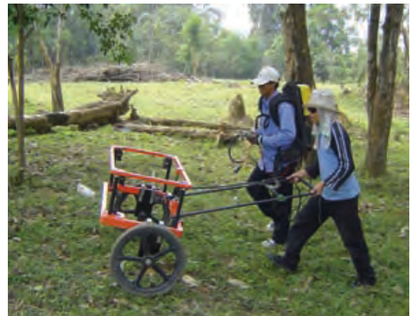
Geophysical Survey With EM61-M2
